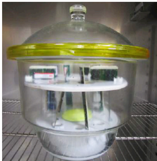
Picture 2: Testing of DRAM modules fitted with anti-sulfuration resistors
