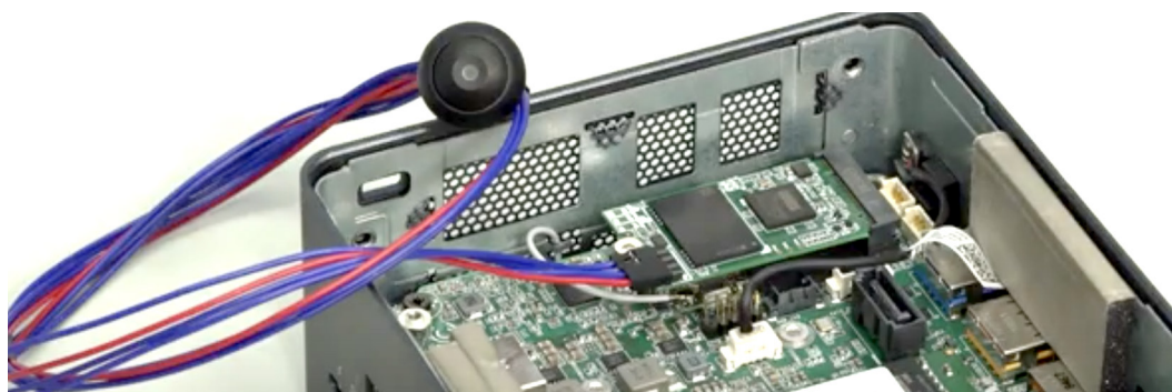
Image 2: An InnoOSR SSD connected to a physical button wire, used for initiating recovery.
