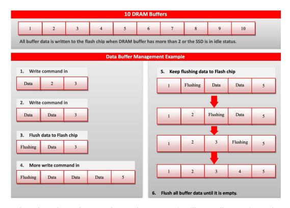
When the voltage detector detects low power, it will stop all operations. The SSD will go into an abnormal power down status. The SSD then writes all data in the DRAM buffer to flash storage. iCell Technology can write up to 15MB of data to flash storage in 60ms.
