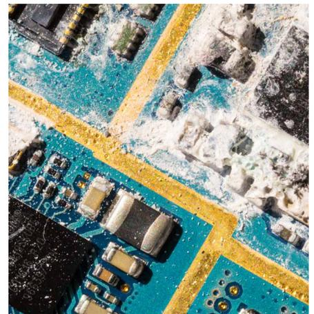
Corrosion will happen as long as an oxidation agent (usually oxygen,  $O_2$ ) is in place. However, once the metal comes in contact with water, electrical conductivity increases and the process speeds up. Any acid will corrode the metal even faster.
