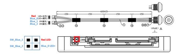
Main feature of InnoOSR family is its OS back up and swift recovery mechanism, which allow field repair easier than ever for malfunction systems with software level damages. As shown in above picture, 2 x 2 pin headers located on the side of standard 7 + 15 pins SATA connector can be used to interact with firmware of InnoInnoAvice to perform OS recovery process and provide LED signal which indicates the recovery status.
