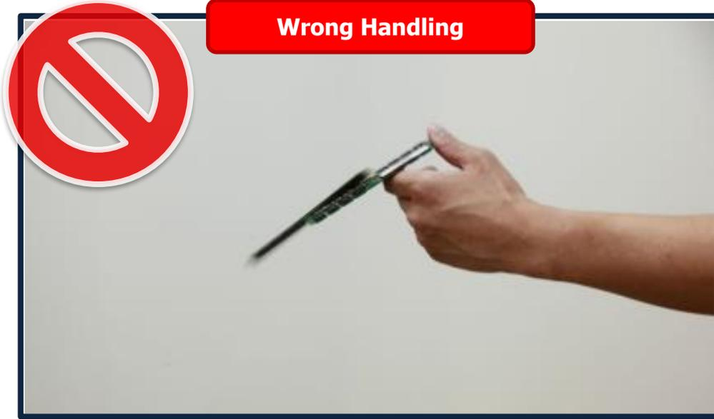
**● Damage Type :**
