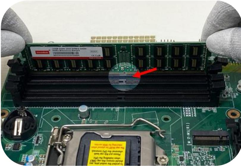
**Align the module notch to the socket.**
