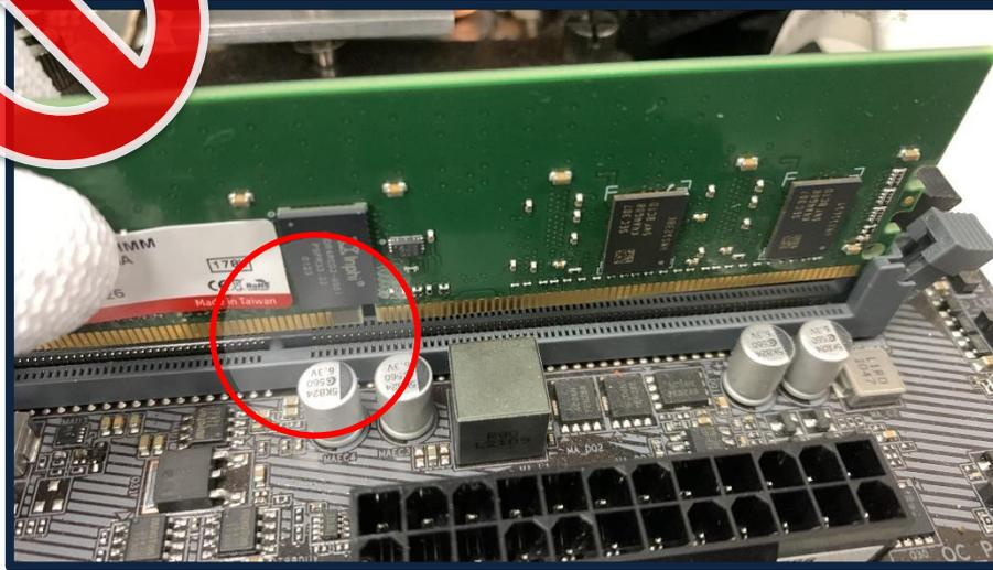
**● Damage Type :**
