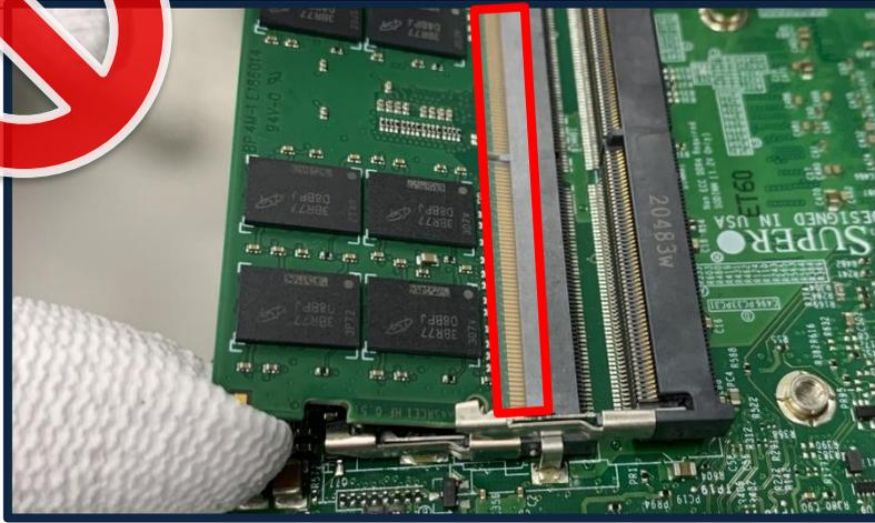
**Do not press module before fully insert.**
