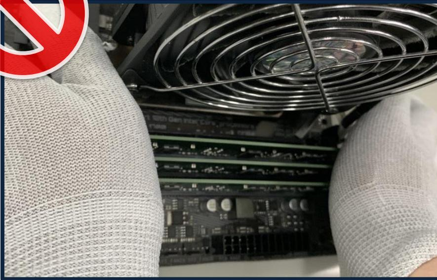
**● Damage Type :**
