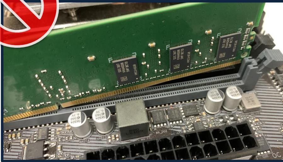
**Do not insert module between sockets.**
