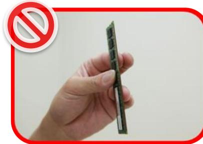
Hold the DIMM using 3 points
