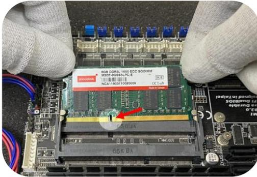
**Align the module notch to the socket.**
