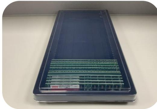
**Tray must be covered with Tray Cover when handling module tray.**
