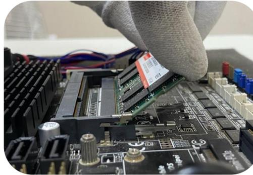
**Hold both sides of the module and insert the module with about 30-degree angle.**
